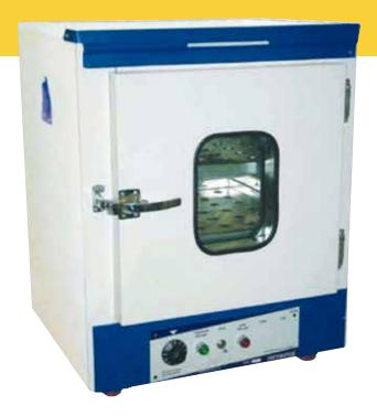
Standard double wall fabrication. Inner chamber made of richly anodized aluminum or highly polished stainless steel sheet and outer made out of thick mild steel finished in white stoving enamel/powder coated paint with mat finished colour combinations. Double wall door with double glass window for observation in the chamber. Temperature range 5°C above ambient to 80°C ± 1°C controlled by a thermostat. The equipment is workable on 220V AC 50 Hz single phase.
