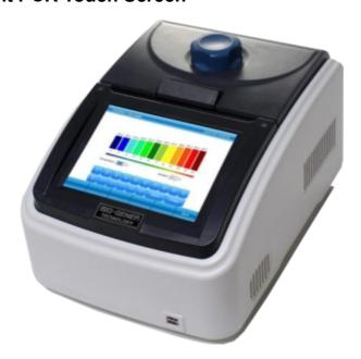
This series product adopts 8 pieces custom-made US Marlow peltier, Max. ramping rate 5°C, cycle times >600000. More advanced technologies applied on the product: Windows operating system; color touch-screen; double blocks can run independently; replaceable block; control by PC function; print function; extra large data storage and USB interfaces. All the above functions make it demand high need experiments.
