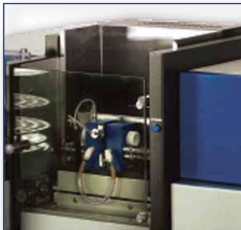
The instrument is equipped with a graphite Furnace Atomiser only. The graphite head is fixed into the optical path to maximise performance and eliminate drift.
